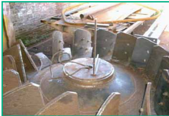
Fan blades protected with Hardplate or Hardlite
