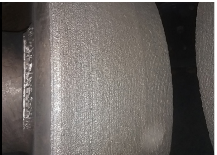
MillCarb™ after 19000hrs grinding
