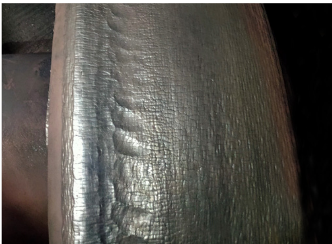
Competitor product after 18000hrs grinding
