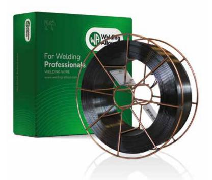
HARDFACE HC-O is a self shielded cored wire with a high chromium cast iron deposit, containing a high proportion of hard primary chromium carbides in a tough austenitic matrix.
