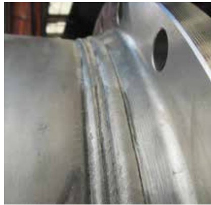
TETRA S 316L-G, flange joining on a pressure vessel
