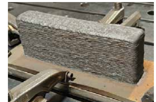
Additive manufactured wall for material qualification of CHROMECORE M 410NiMo-G
