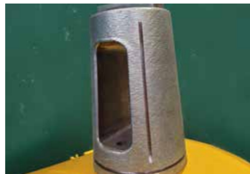
Cladding of a plug valve using STELLOY 6-LD
