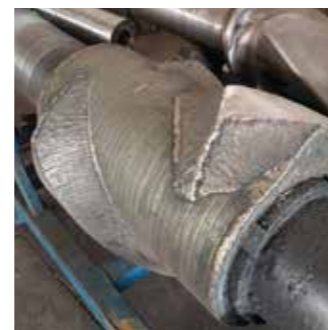
Rubber mixer hardfaced with STELLOY 6-G
