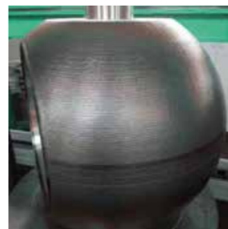
Ball valve hardfaced with STELLOY 6-TIG
