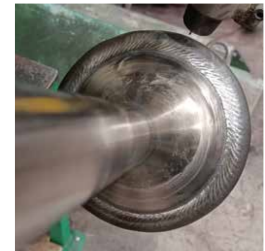
Exhaust valve seat hardfaced with STELLOY 6-G
