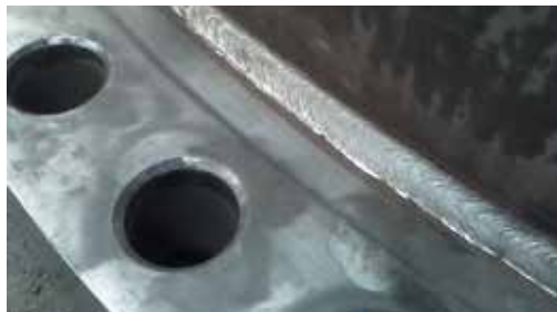
Flange welded with TETRA S 22 9 3L-G.
