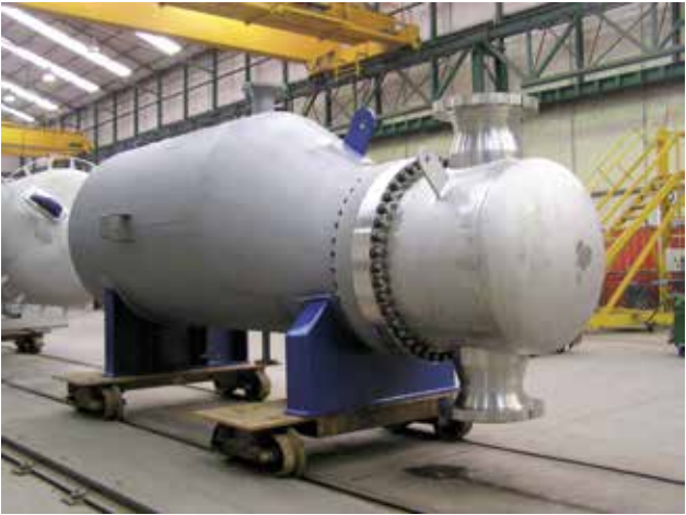
High pressure reboiler in SS 316L.
