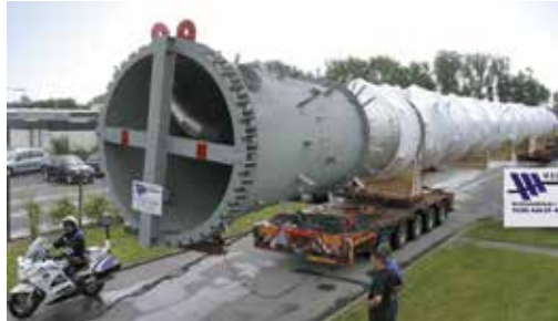
Hydrolyser column in duplex stainless steel.
