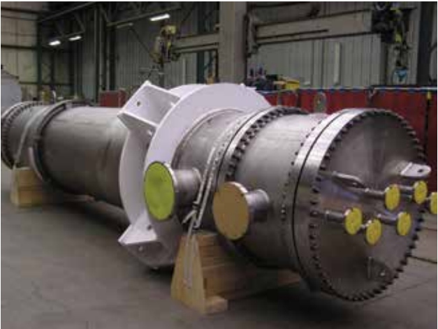
Gas cooler in duplex stainless steel.
