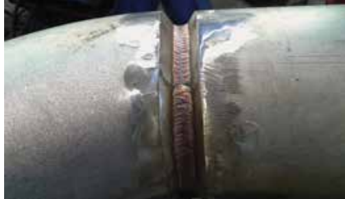
Tube welded with TETRA V 317L-G.
