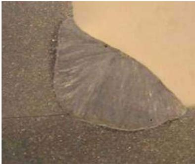
Figure 4 shows a PB-2F fillet weld on AISI 310. The characteristic convex shape of the basic flux cored wire fillet favours a reduced tendency to hot cracking.
