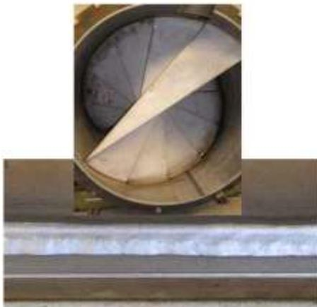
Figure 7 Horizontal fillet weld in AISI 304H using TETRA S 308H-G (E308HT0-4) – a typical application for stainless steel flux-cored wire with slow freezing slag
