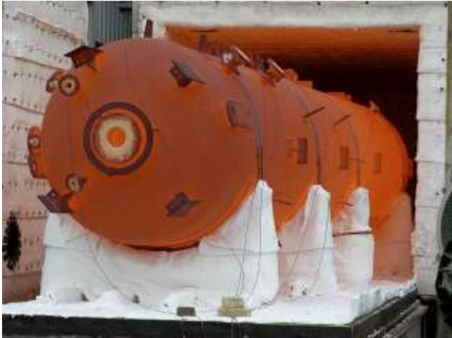
Figure 11: 310S reactor under heat treatment
