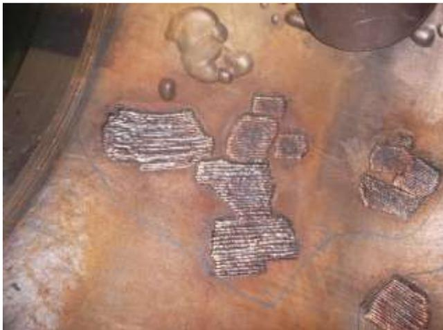
Figure 12: Repair of casting defects on
