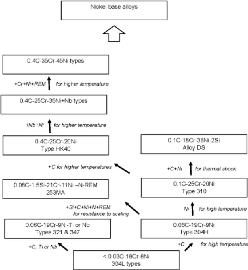
Figure 5: stainless steels designed for service at high temperature (from J.C.M. Farrar) [2].
