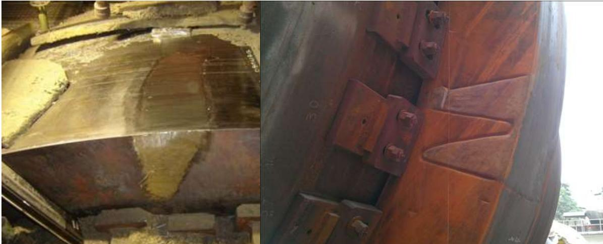
Figure 13: Crack repair with nickel base bismuth free wire GAMMA 182 (NiCrFe-3), as welded and after 30 months service life
