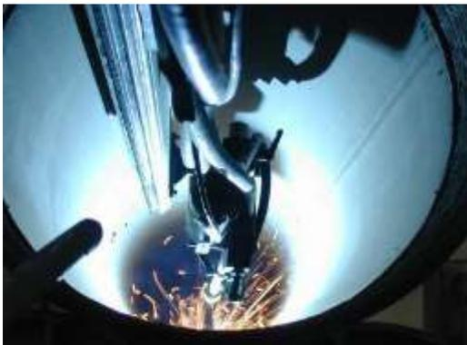
Self-shielded stainless steel wires are of interest for cladding and repair work, and small diameter wires are also used for assembly work when the use of an external gas protection is impractical or uneconomic.
