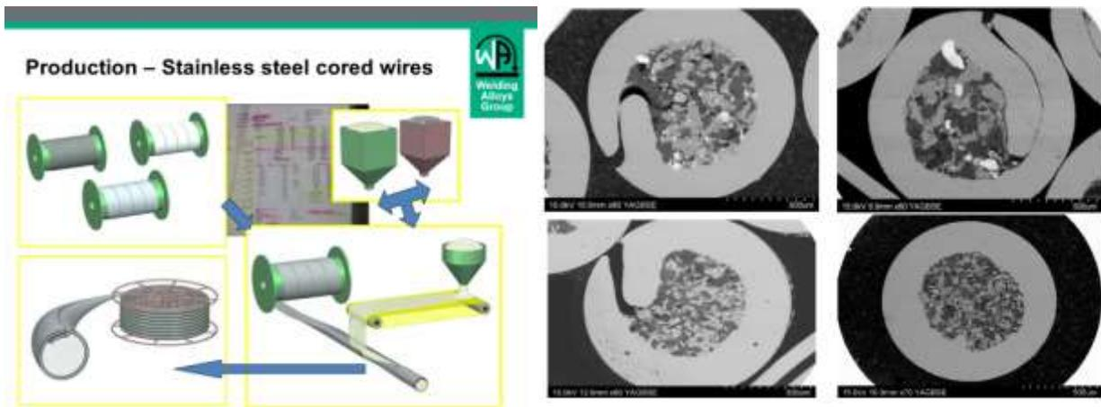
Figure 2: left side; production route – right side; typical modern seam configurations for 1.2 mm wire
