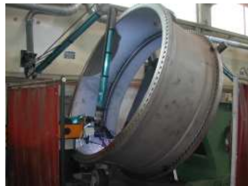
Figure 14 GMAW cladding with STELLOY 21-G
