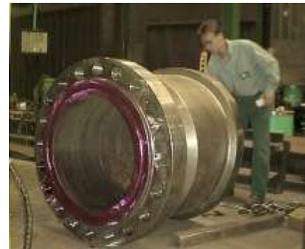
Figure 2: GMAW with TUBE S Two layer 904L cladding
