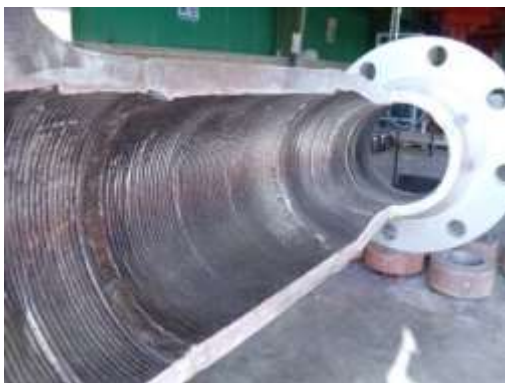
Figure 13 Internal cladding of grit traps with STELLOY 6-G
