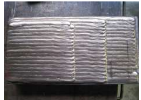
Figure 5: TUBE S 904L-S, weld appearance
