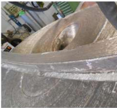
Figure 6: Cladding with Bi-Free cored wires Layer 1: TETRA V 309LNb-G Layer 2: TETRA V 347L-G
