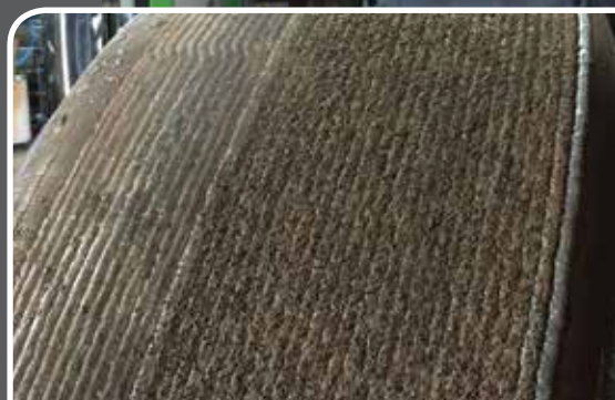
Vertical mill tyre welded with standard hardfacing on the left and MillCarb™ on the right
