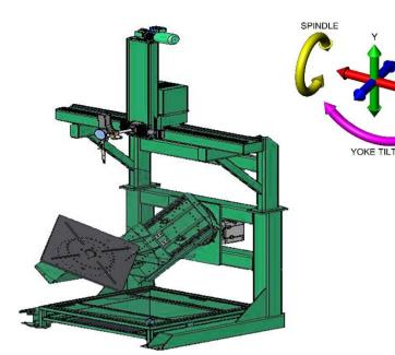
Automatic machine with component rotation via the spindle arm and yoke and manipulation in linear axis X, Y and Z including wirefeed system. Component is supported and attached on the face plate of the Headstock. Fully automated via the integrated control system and motor drives
