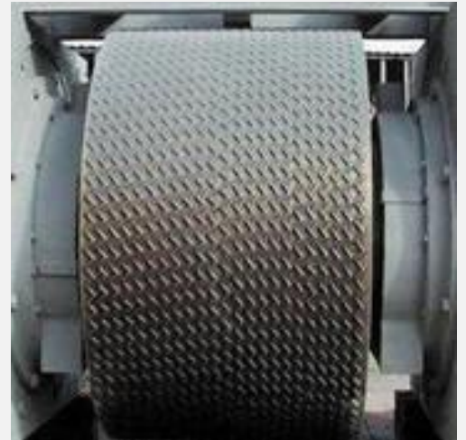
Typical appearance of a Roller Press Roller after refurbishment with the inlay as proof of the crack resisting properties of the buffer layer.
