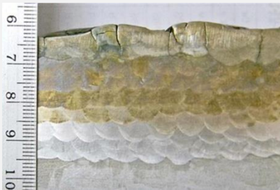
Stress relieve cracks do not propagate into the buffer layer.
