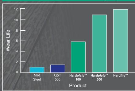
The graph reflects results from the ASTM G-65 wear test performed by an independent laboratory.
