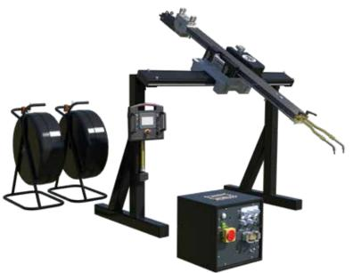
The Sugar Mill Kit (SMK) is a portable welding machine designed to weld crusher rolls used in the sugar industry. With this lightweight piece of automated equipment, you can carry out arcing, rebuilding and teardrop welding of the sugar rolls to optimise crushing efficiency and prolong service life. The machine can also be used for welding other components used in sugar mills, such as trash plates.
