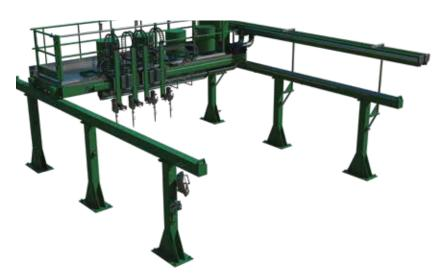
This automated Flat Plate Cladder offers a turnkey package for the manufacture of hardfaced plates, combining weld assembly, tables and an easy to use control system. It can be configured to suit the scale of your welding requirements, from using a single welding head to multiple heads, for cladding of a single plate or two plates simultaneously.
