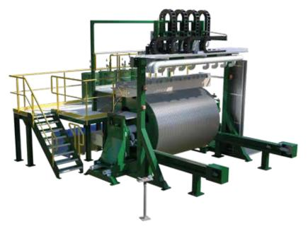
The Rotary Plate Cladder is a heavy-duty machine designed for automated welding of plates. It can be equipped with multiple welding heads, which are set-up to continuously hardface plates that are mounted on a drum up to 8 tons.
