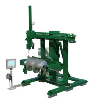
Screwflight is designed to clad the different parts of a screw, in all positions allowing welding in the downhand position and with very impressive production speeds.
