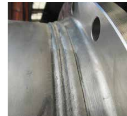
TETRA S 316L-G, flange joining on a pressure vessel
