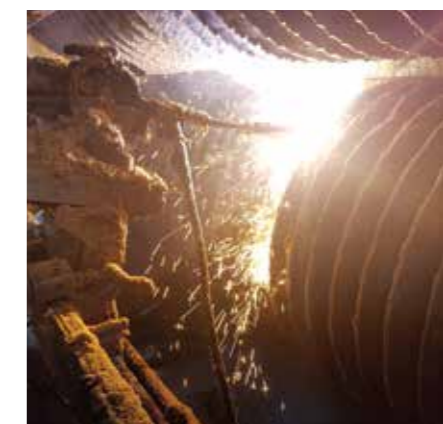
Sugar: repair and refurbishment of rolls
